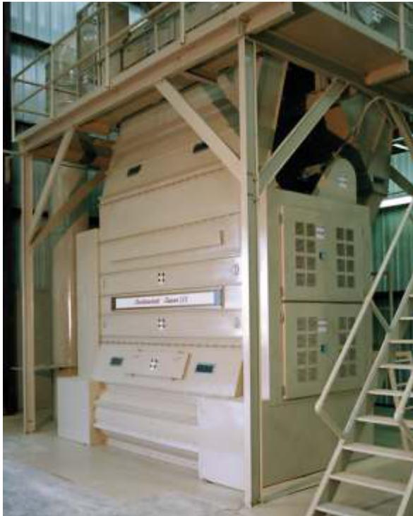
Inclined Cleaner over the Super III Stick machine with a 36" vacuum.
